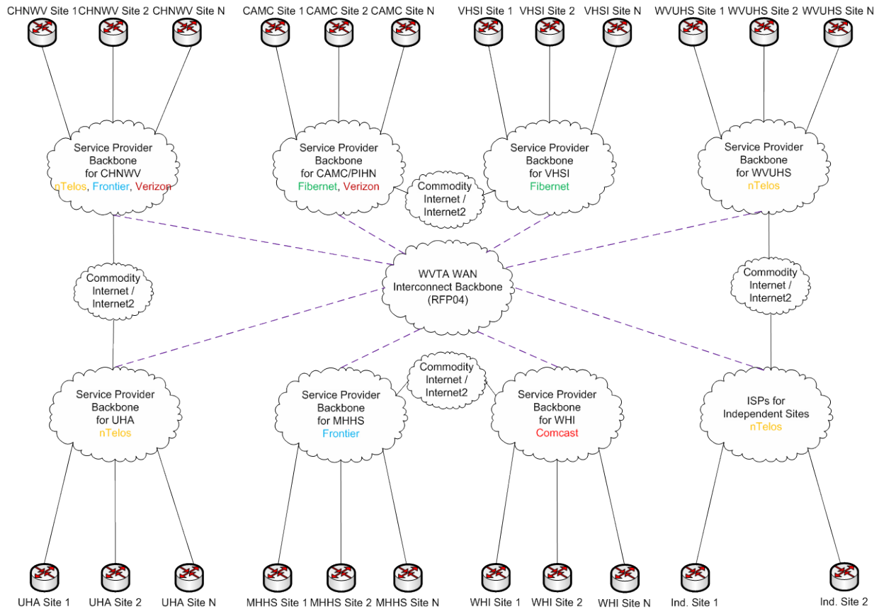
Figure 1: WVTA WAN Hub Interconnect High Level Topology (Source: WVTA)
